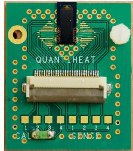
This new membrane device provides two modes of spatially localised sample heating up to 100°C and an absolute noise thermometer for monitoring the sample temperature as it is interrogated by the SThM tip. By measuring the probe response in and out of contact, in different heating modes, and at different temperatures, one can quickly and accurately calibrate the SThM temperature sensor with a few mK accuracy.
