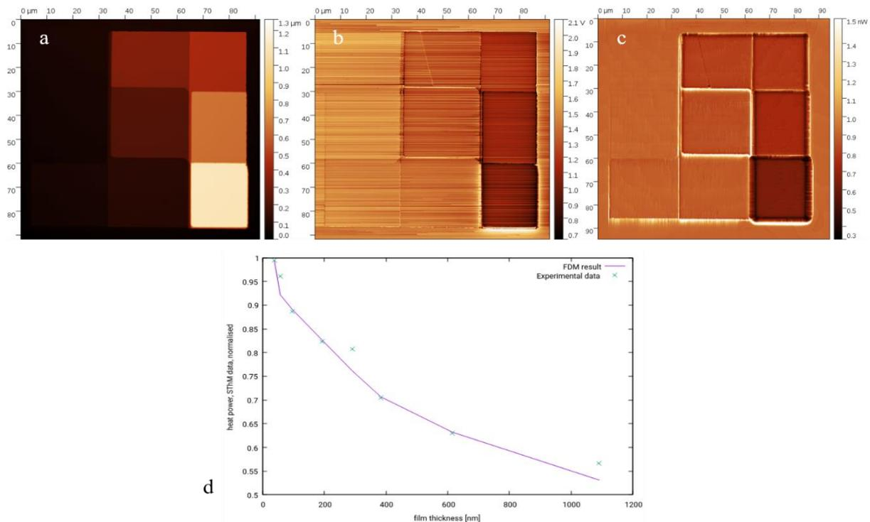
Figure 2: (a) Topography, (b) Thermal data, (c) Modelled SThM data and (d) showing the normalised data from (b) and (c) against the step thickness<sup>1</sup>
