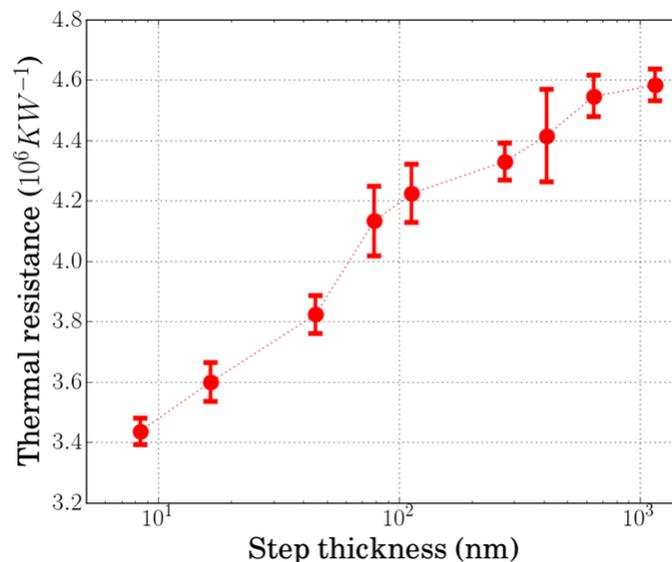
*Figure 3: Thermal resistance at the probe apex measured as a function of step thickness of oxide sample (at ULANC).*
