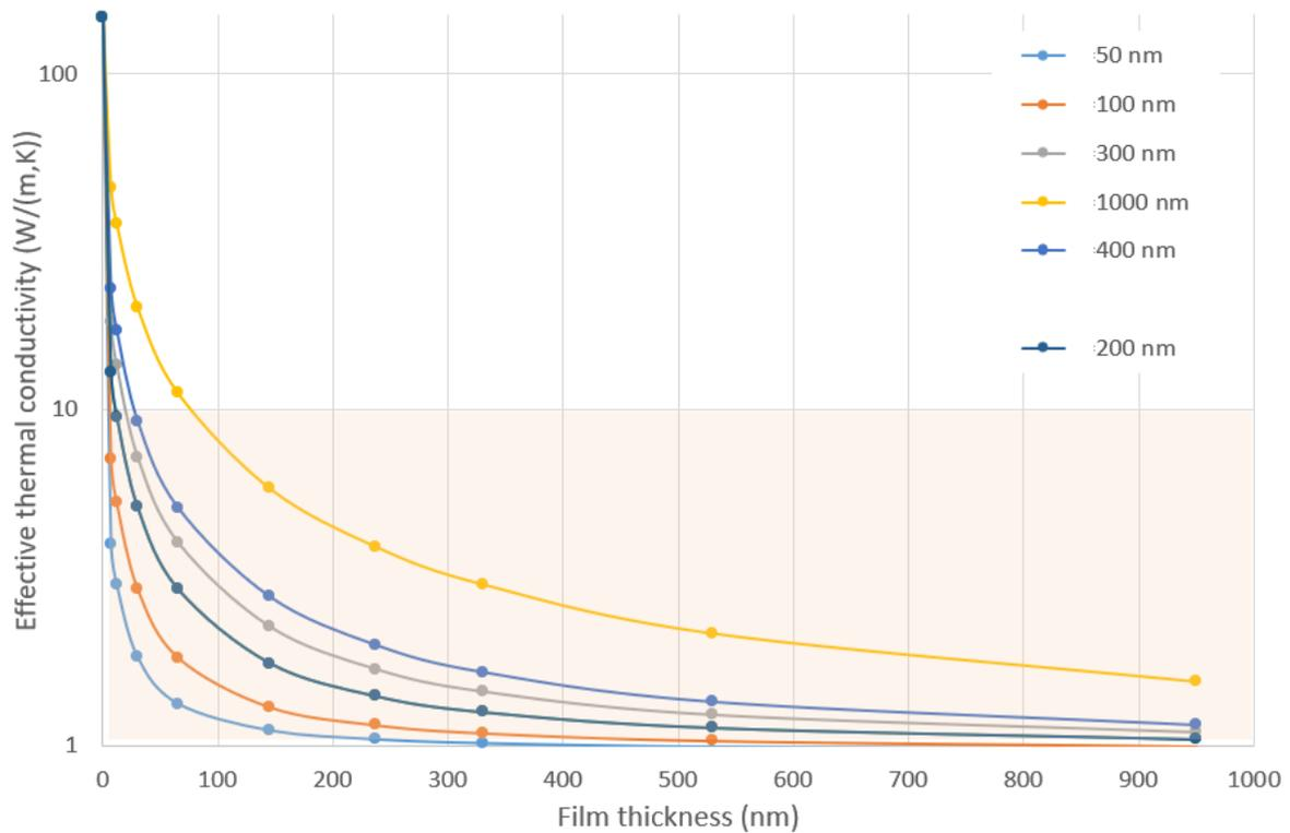
Figure 4: Modelled effective thermal conductivity of the oxide sample as a function of thickness for tips with effective contact radius 50nm – 1000nm
