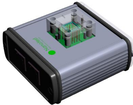
Figure 5: CAD-drawing of chip holder with spring probes connecting the chip to RJ45 connectors.
