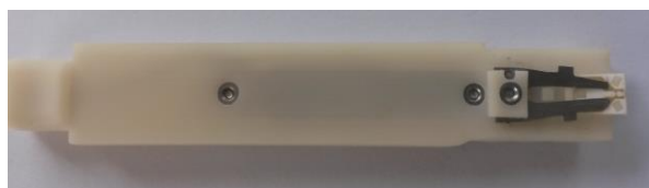
Figure 3: Probe holder with 2 terminals
